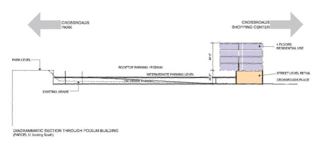
There is a significant grade change at the East edge of the property where it abuts Crossroads Park. This offers the opportunity to build two-story parking structures (with minimal excavation costs), the upper level of which would match the ground level of the park. This makes it very feasible to construct 'podium buildings' for residential or office uses that could feature:
